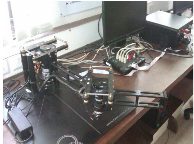
Fig. 2 Quanser serial flexible joint set-up
